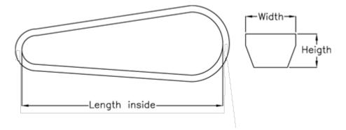
$\begin{array}{ll} \text{Datum Llength} = 550 \\ \text{Height} & = 6 \\ \text{Length inside} & = 530 \\ \text{Width} & = 10 \\ \end{array}$
